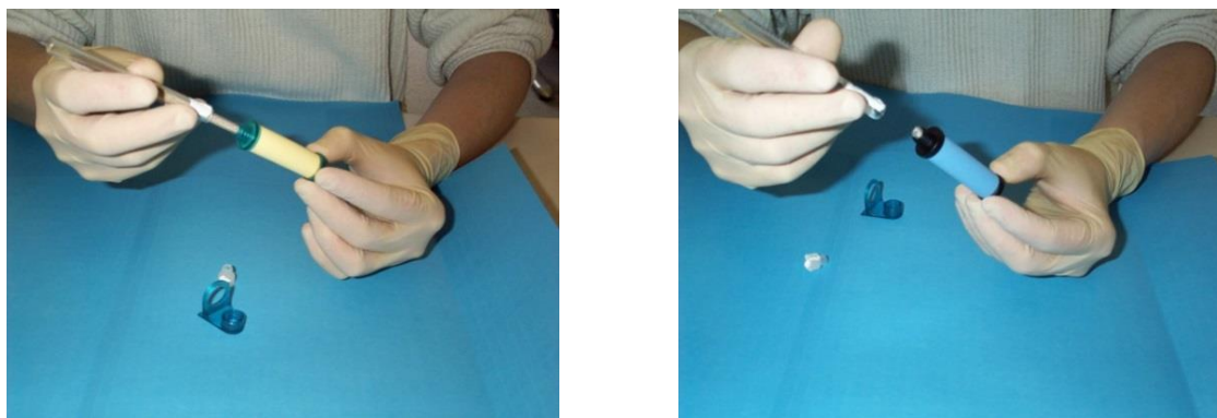
Figure 1. Procedure to set up the Radiello® samplers
