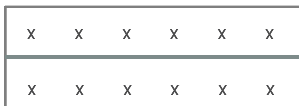
Figure 6. Selection of different points to measure air velocity
